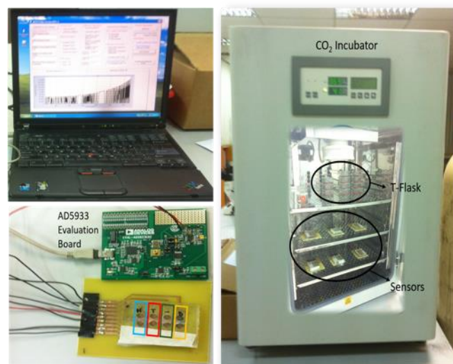
Fig. 2 Right- Sensors and T-flask positioned inside incubator. Left- Impedance and phase measurement were taken using AD5933 evaluation board and laptop. Four sets of double experiments were conducted on a single board; cell+natural product (blue box), cell+taxol (red box), cell+DMSO (green box) and control cell without drugs (yellow box).
