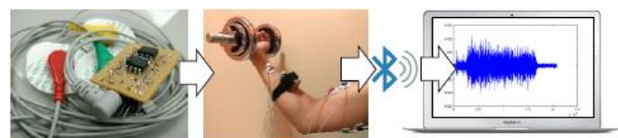
Fig. 4: Hardware architecture of sEMG device
