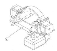
**Fig. 2** Illustrated an embodiment of the Wrist-T device. The details of hand support include a). palm rest and finger rest; b). vertical hand grip stand; and c). horizontal hand grip stand. Notes: Description of the reference numerals used in the accompanying drawings according to the WRist-T device; (1) channel; (2) platform arm; (3) motor; (4) hand support; (5) controller; (6) toggle switch; (7) power button; (8) LCD display.
