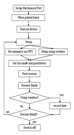
Fig. 3 The flowchart of the WRist-T device function.
