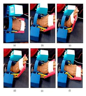
**Fig. 6** A 3D printed proof-of-concept prototype of WRist-T device tested by a stroke patient. The (a-f) shows details the example wrist of motion on extension exercise.
