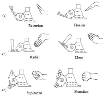
**Fig. 4** A perspective views of the device in an embodiment to give a). flexion and extension; b). radial deviation and ulnar deviation; and c). supination and pronation of the wrist.
