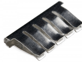
Figure 4. A single strip of conductive metal removed from the above breadboard [1].
