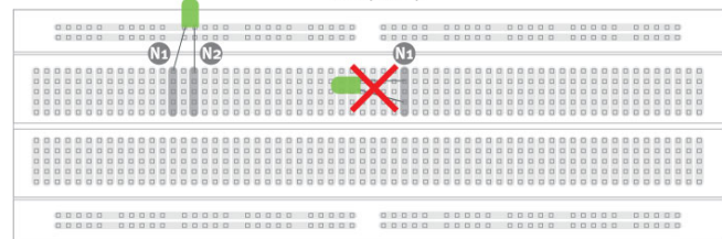
Figure 14. Put different legs of LEDs on different columns [5].
