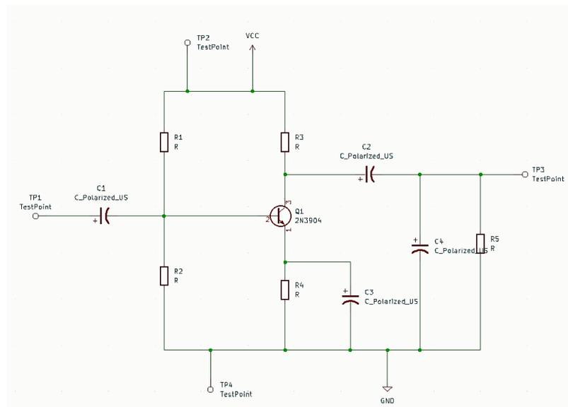
Figure 1: Example of small signal amplifier circuit
