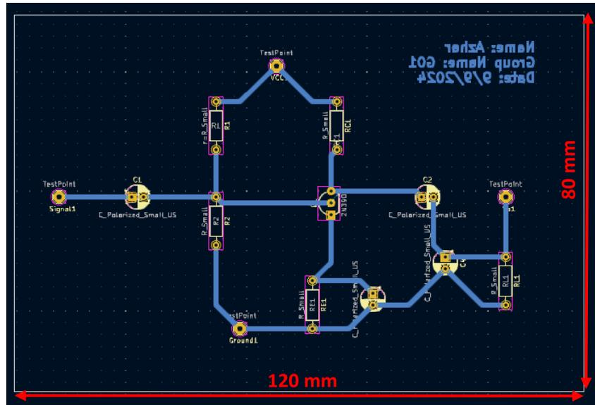
Figure 2: Example of PCB layout design for small signal amplifier circuit
