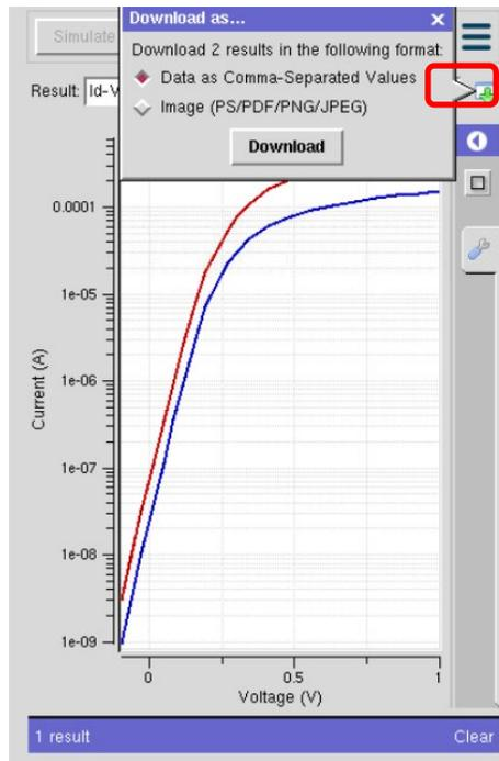
16. Analyze the electrical parameters. From the Log  $I_D$ - $V_G$  plot, ( $V_{D1} = 0.05V$  for linear region and  $V_{D2} = 1.0V$  for saturation region).
