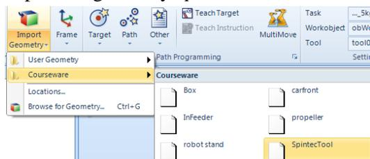
*A geometry representing the tool is now imported to the station and placed with its local origin in the zero point of the world coordinate system. As the local origin on this specific part is not placed in the attach point of the tool you will see the offset between the coordinate system and actual CAD part.*
