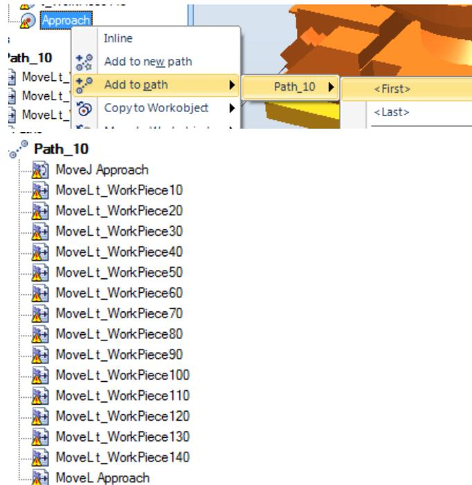
6. Run Auto Configuration to set the axes configurations. Either from the context menu of the path or the **Modify** tab.
