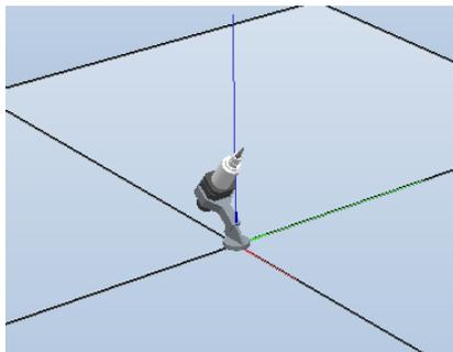
9. Attach the tool geometry to the robot to see the difference. Now it should attach correctly.
