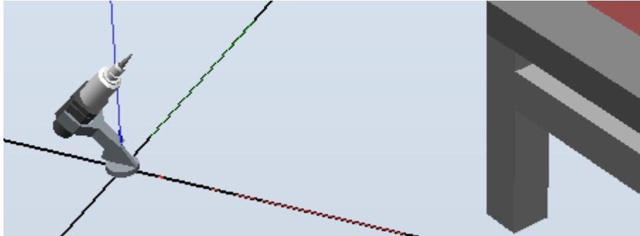
Click in the Graphics to remove the red marking and the robot will now be invisible and you can see the tool on the floor. In the Layout browser the node for the robot is marked with a magnifying glass
