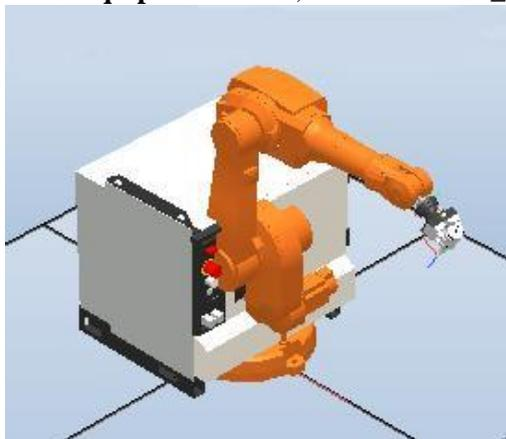
*The cabinet will be imported to the station and placed at the origin of the world coordinate system.*
