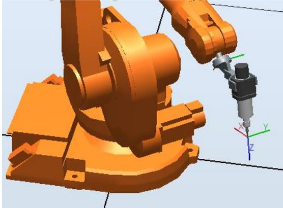
*The tool is attached to the flange of the robot.*
