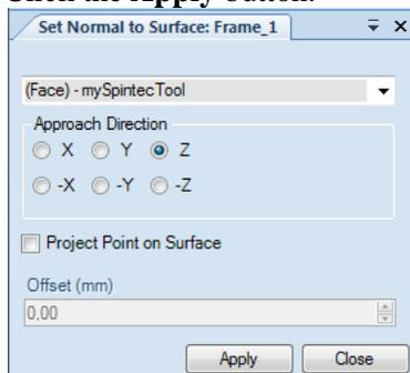
Since the default definition of the approach direction is positive Z it points out of the surface.
