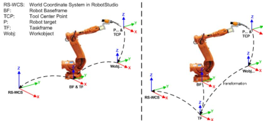
Here you can see how a task frame in RobotStudio environment is mapped to the robot controller coordinate system in the real world, e.g. in a shopfloor.
