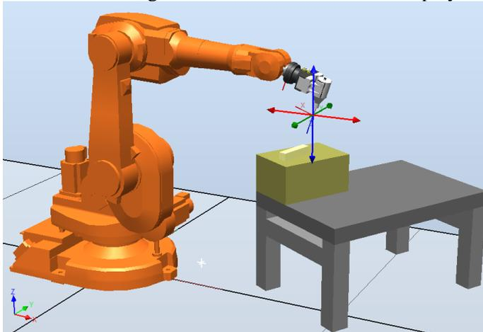
3. Click and drag the arrows to jog the robot. Use the red arrow for X direction, green for Y and blue for Z.
