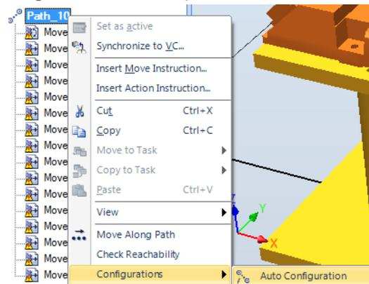
7. As configuration for the first target, select (0,0,-1,0). Press **Apply**. Now the configurations for the rest of the targets are calculated.
