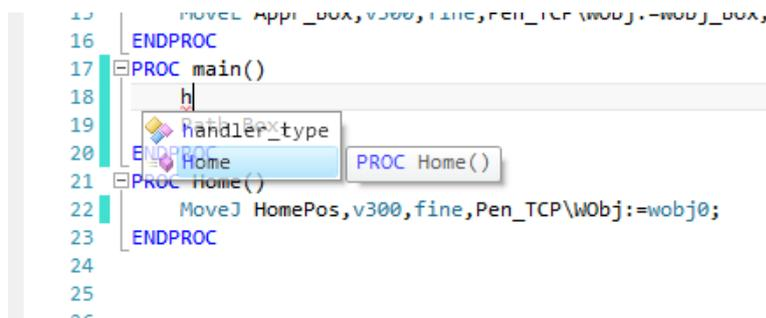
Note the IntelliSense as you start to type. The return key will add the highlighted instruction/procedure.
