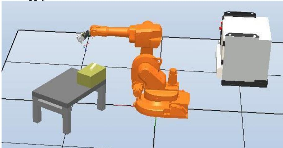
The primary point on the box is now moved to the primary point on the table and the points on the X-Axis set the orientation of the box.
