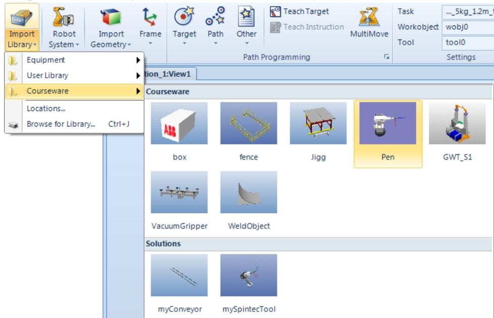
*The tool will be imported to the station and placed at the origin of the world coordinate system, thus hidden inside the robot. However, in the Layout browser you can see that the tool has been imported.*
