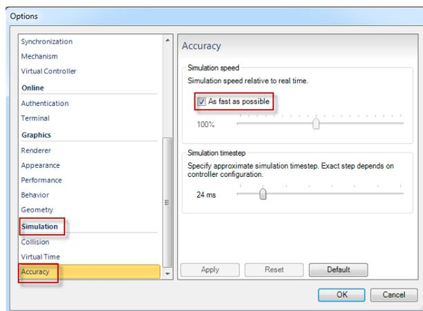
4. Press **Play** from the **Simulation** tab to run the simulation again. Now note that it will run through the simulation in a much shorter time but the resulting process time will be the same.
