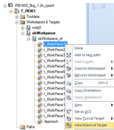
2. As all targets seems to be possible to reach, de-activate **View Robot at target** again.
