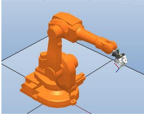
*The tool is moved to the wrist of the robot.*
