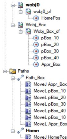
19. To transfer the new instructions to the virtual controller, click **Synchronize to VC** from the **RAPID** tab.
