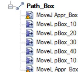
Note that the yellow triangle warning appears on the new instructions. This is because no axes configuration is set yet.
