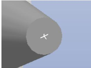
The snap goes to the center of the surface as our selection level and snap mode.
