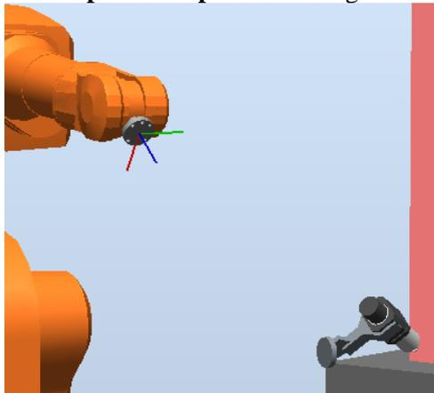
*Due to the definition of the local coordinate system of the part, you get an offset of the tool. This is what we now have to fix.*
