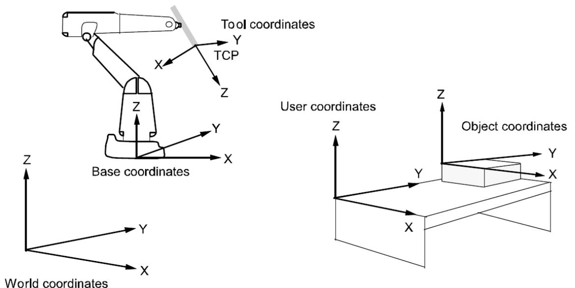
A workobject consists of two frames. The **User Frame** (User coordinate system) is referenced from the **World Coordinate System** and the **Object Frame** (Object coordinate system) is
