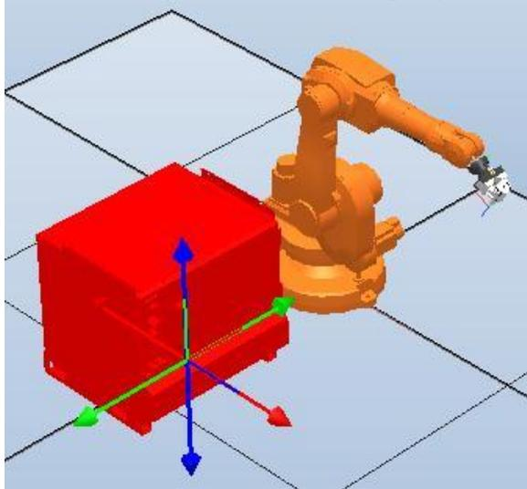
4. Click and hold on the green arrow in the Freehand move cross, then drag the controller one floor square (about 1 meter) to the right of the robot (negative Y direction). Then click and hold on the red arrow and drag it one square backwards (negative X direction).
