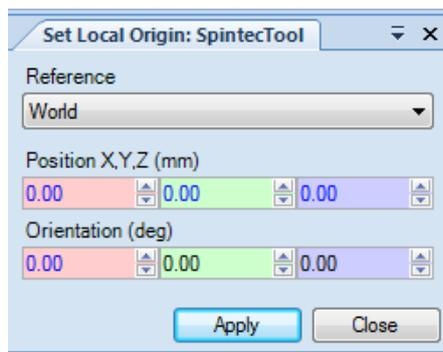
*The coordinate system is now moved to coincide with the actual position in the station which also happens to be the attachment point of our tool geometry.*
