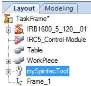
*In the Layout window we can see that the geometry part has been replaced by the tool mechanism. But that the frame remains.*
