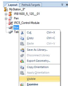
Next step is to set a suitable configuration on the first target and then re-use this orientation for the rest of our targets. If the exact orientation is known, it is easiest to manually type these values into the **Set Position** dialog. In this case when we have no exact values we will manually adjust the orientation of the first target.
