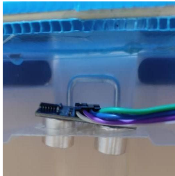
Figure 16: Ultrasonic sensor stick on the Top of Dustbin Lid for Measure the Level of Garbage
