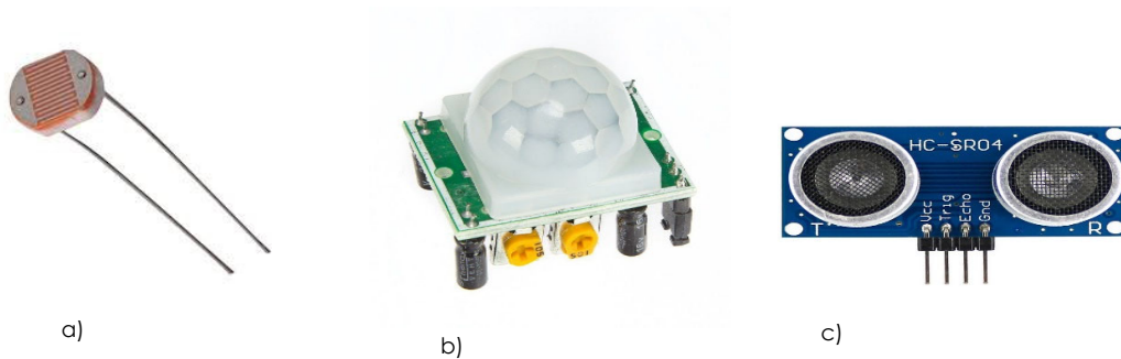
Figure 6: a) LDR b) PIR motion sensor c) Ultrasonic sensor HC-SR04
