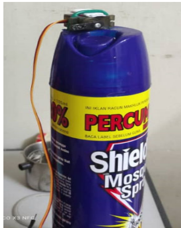
Figure 14: Attached servo motor on aerosol can
