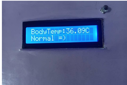
Figure 23: Displaying the body temperature on I2C LCD.
