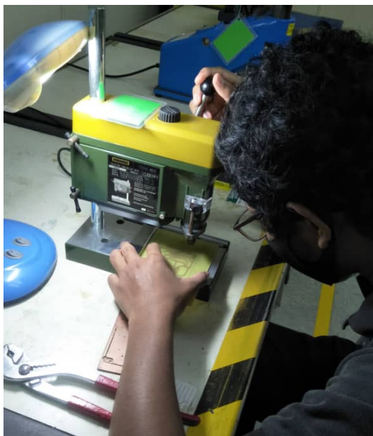
Figure 14: Drilling PCB process
