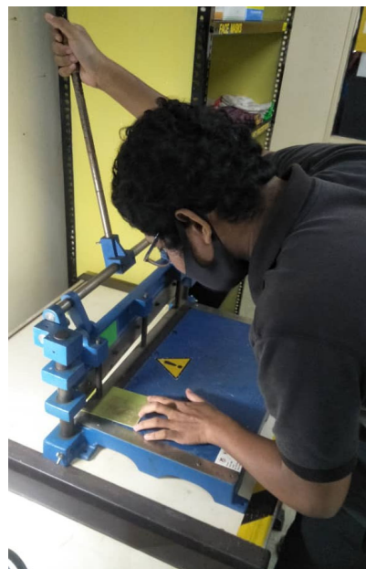
Figure 15: Cutting PCB process
