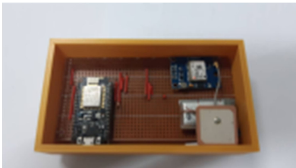
Figure 14: 3D printed casing for the electronic hardware
