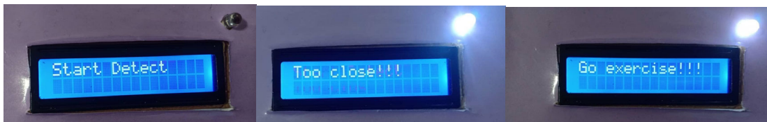
Figure 19: Message display on LCD for ergonomic function.
