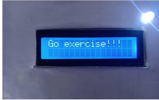
Figure 26: Displaying a reminder to the user on I2C LCD.
