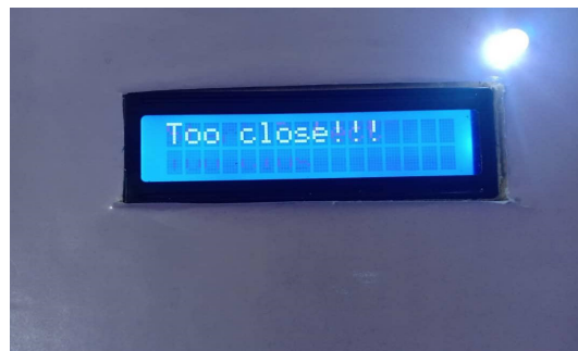
Figure 25: Displaying an alert message to the user on I2C LCD.
