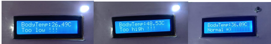
Figure 18: Body temperature display on LCD.
