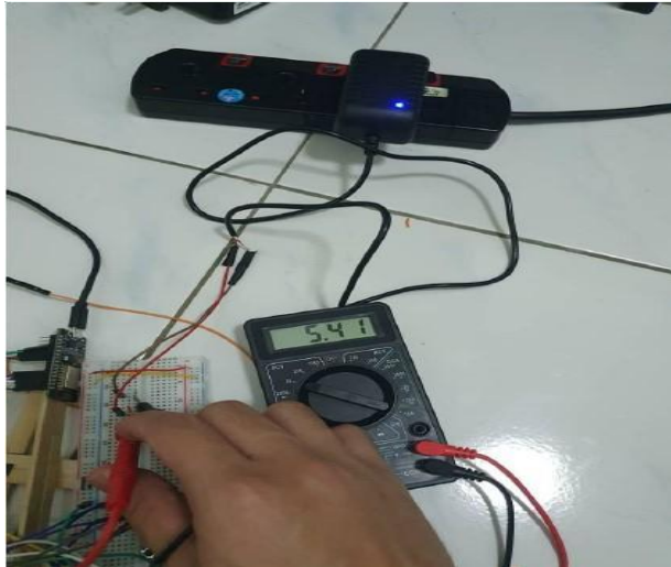
Figure 24: Test of Voltage Output from 5V Adapter without Voltage Regulator
