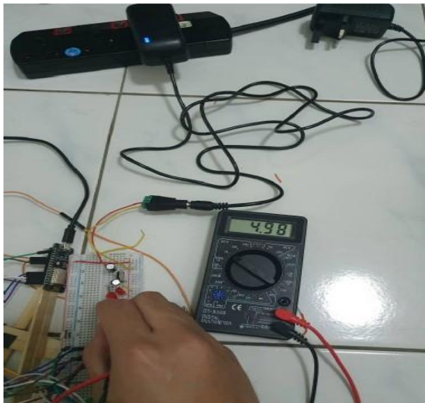
Figure 25: Test of Voltage Output from 12V Adapter with Voltage Regulator
