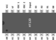
Figure 28: HT12D Radio Frequency Decoder pinout
