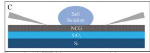
Figure 2: Cross-sectional view of the NCG strip fabricated [8].
