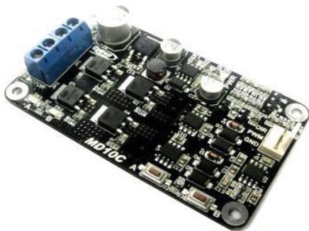
Figure 3: MD10C motor driver
