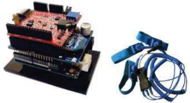
Fig. 5. Wireless ECG acquisition unit with passive electrode
