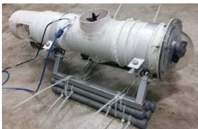
Fig. 9. Full ROV design
