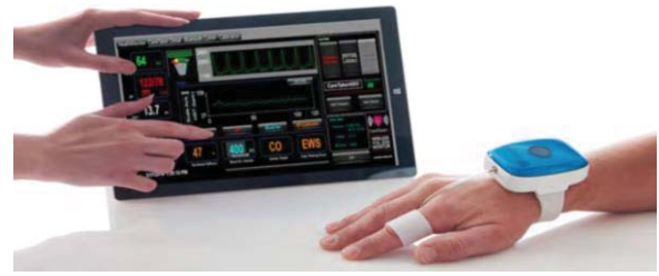
Fig. 3. Wireless continuous non-invasive "beat-by-beat" blood pressure and heart rate monitor [4].
