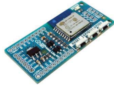
Figure 4 ESPresso Lite V2.0
