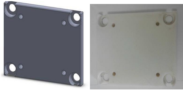
Fig.6 Precision positioner holder in SolidWorks and after it fabricate to 3D
