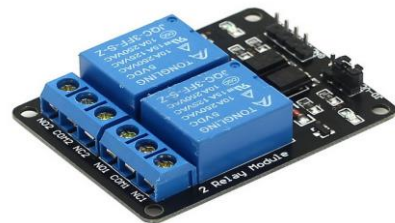
Fig 9: 5V Two 2 Channel Relay Module with Optocoupler
