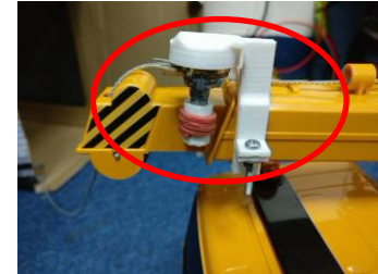
Fig. 4 Potentiometer to measure boom length
