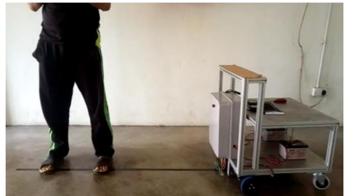
Figure 7 : Obstacle Avoidance Testing work setup
