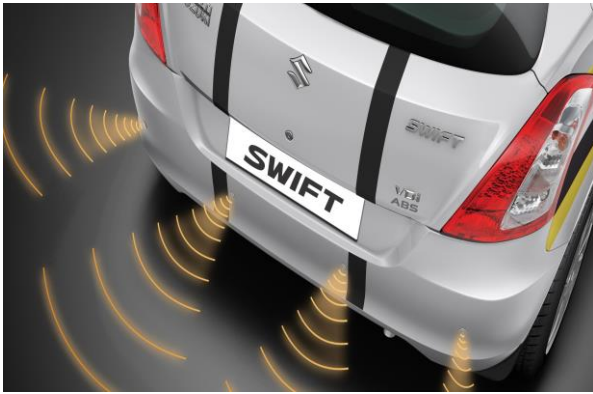
Fig. 1. Reverse Parking Sensor System on Suzuki Swift
