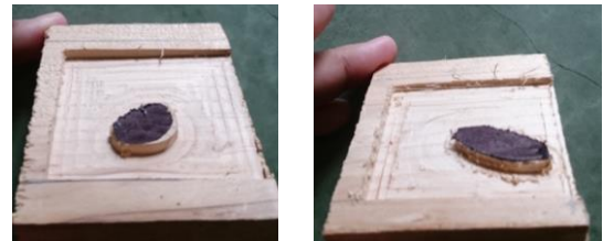
Fig. 9. Sample result after carving 1mm depth.
