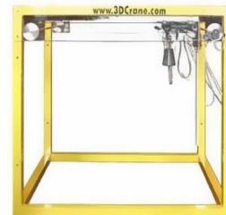
Fig. 4. An Overhead crane system by INTECO
