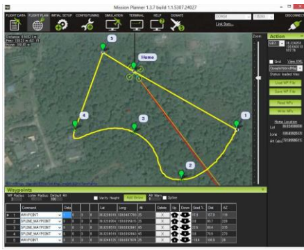
Fig. 11. Assign the waypoint for the quadcopter using Mission Planner
