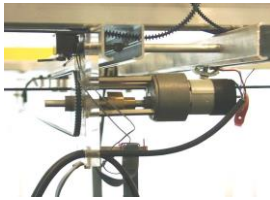
Fig. 8. Motor drive of the overhead crane system
